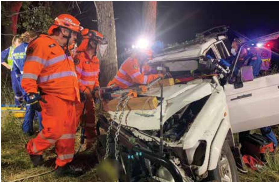
SES rescue operators the setting up of the hydraulic equipment for 'dash roll'
