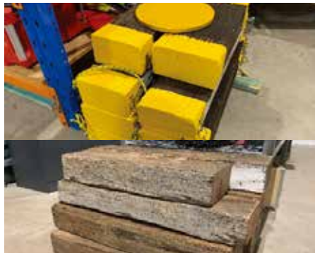
Our heavy timber, hardwood cribbing blocks. They were cut, oiled and painted to help preserve them and fitted with rope carry handles for ease of movement. The metal base plate for the ram can be seen lying on top of the timber.
